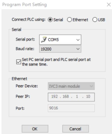
Figure 3.2 Serial port setting for program download
