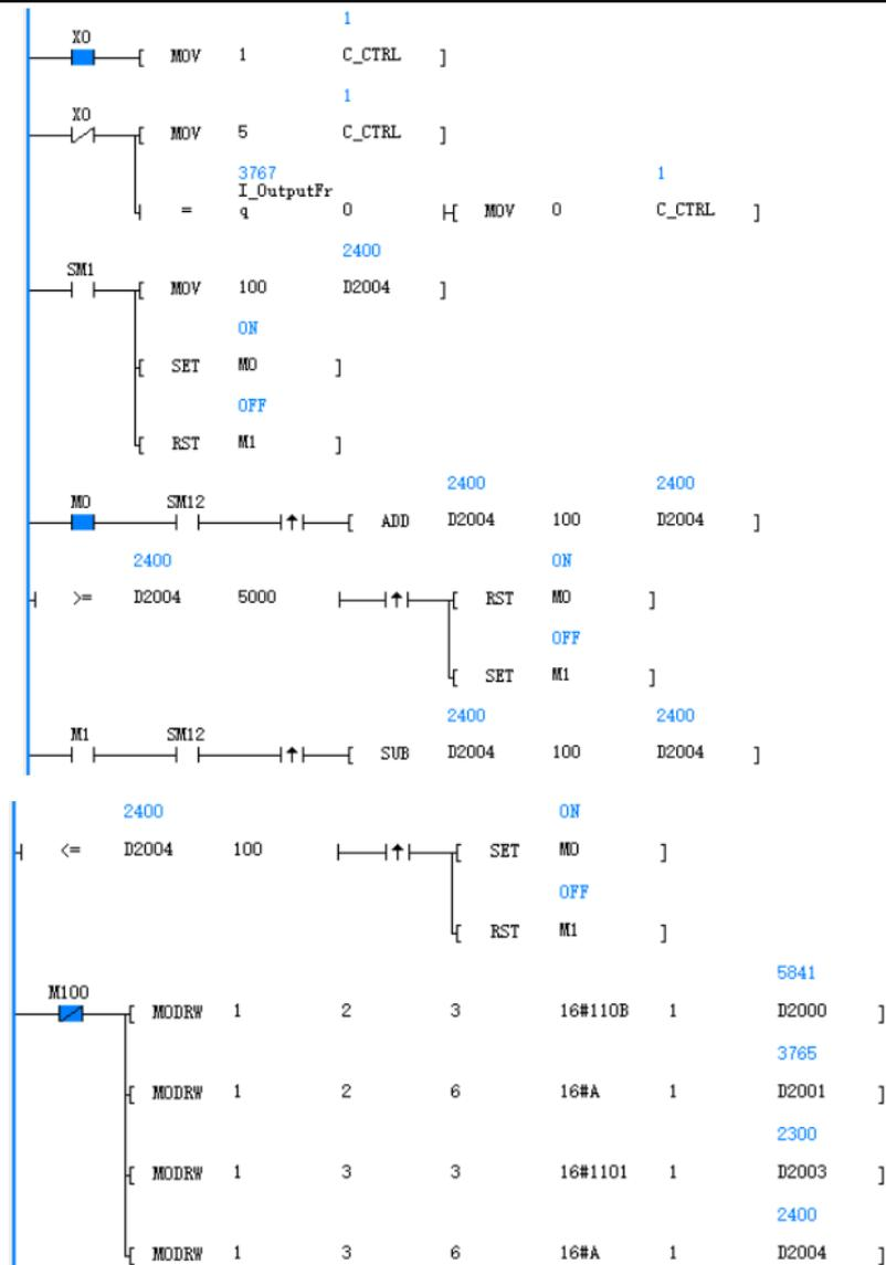
Figure 5.6 Programming case for RS485 communication
