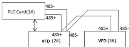
Figure 5.5 PLC card networking example
